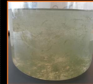
Figure 4: Praestol A 6291 flocculant added to Western Wastewater causes distinct flocculation
