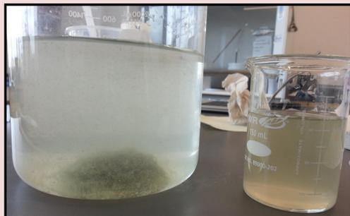
Figure 1: Left: Western Pulp wastewater that has been treated with Praestol A 6291; Right: untreated Western Pulp wastewater
