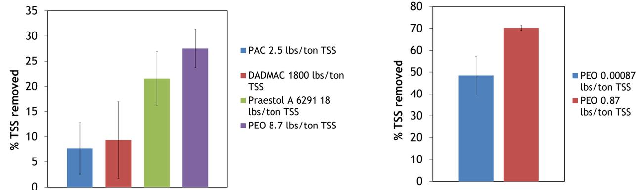
Figure 2: TSS removal on Western Pulp wastewater using various flocculants. Dosages are based on the amount of suspended solids in the wastewater. The most successful flocculant to date is polyethylene oxide (PEO), with 27% removal.
