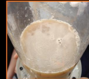
Figure 5: PEO flocculant added to Stimson wastewater creates a foam during flotation
