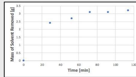
Figure 3: The mass of solvent removed over time at 140°C when loaded with 6.7 grams of solvent.
