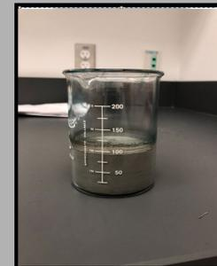
Figure 9: Powder and solvent were added to a beaker and the mass was recorded. The mixture was taken out and the mass was measured at 20-30 minute intervals for up to 4 hours.
