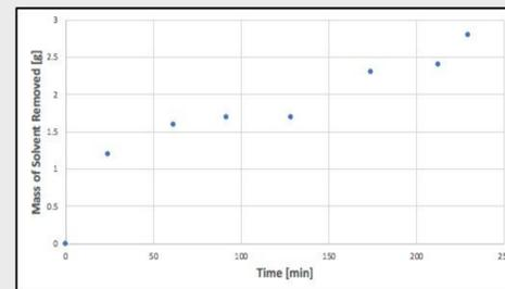
Figure 5: The mass of solvent removed over time at 140°C when loaded with 6.4 grams of solvent.
