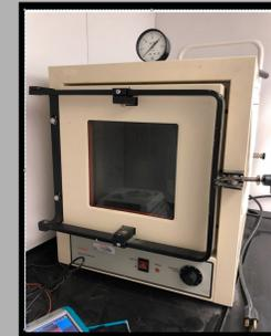
Figure 8: Vacuum oven that was used to conduct flux experiments for solvent transport. The vacuum oven was set at 140-150°C. Both the solvent and powder were preheated before mixing and experimentation
