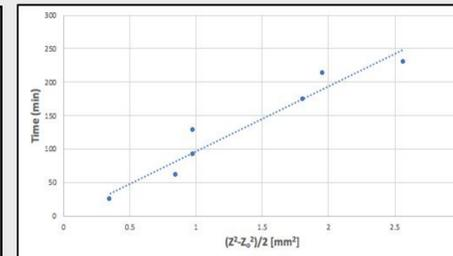
Figure 4: After plotting the Arnold Model pathlength vs time from Eq. 1, the Diffusion Coefficient,  $D_{AB}$ , was able to be estimated from the slope to be  $0.01 \text{ cm}^2/\text{s}$ .
