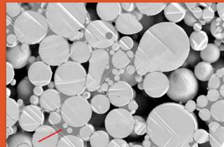
Figure 2: Microscopic scale picture of solvent within the powder pores.
