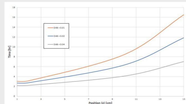
Figure 7: The time required for 6.4 g of solvent to be completely removed at a designated position away from the part,  $z$ , at diffusion coefficients of  $0.01, 0.02, \text{ and } 0.04 \text{ cm}^2/\text{s}$ .
