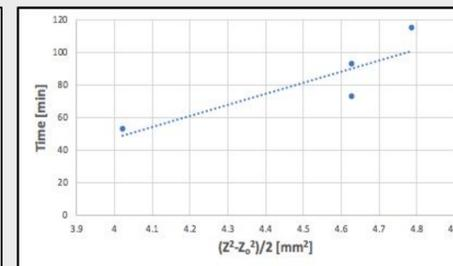
Figure 6: After plotting the Arnold Model pathlength vs time from Eq. 1, the Diffusion Coefficient,  $D_{AB}$ , was able to be estimated from the slope to be  $0.02 \text{ cm}^2/\text{s}$ .
