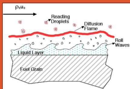
Figure 2: Melt layer diagram of the liquid solid interface.
