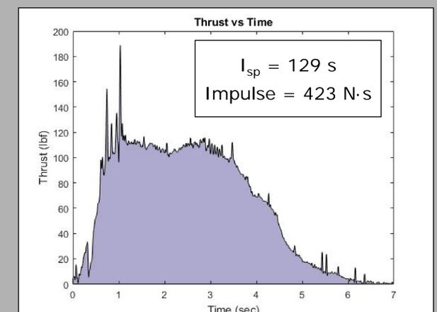
Figure 8: The thrust curve given by the load cell (shown in Figure 5) for the composition of 25% Al, 10% cornstarch, 2% carbon black, 63% paraffin.
