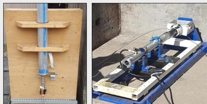
Figure 3: Sub-scale testing setup includes a nitrous holding tank as well as the subscale motor on the thrust sled.
