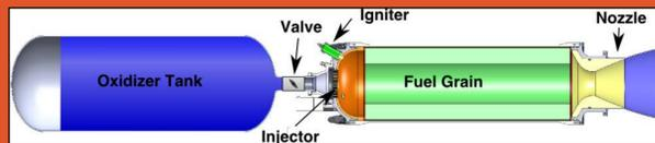
Figure 1: Standard hybrid rocket propulsion system with oxidizer tank, fuel grain, and exhaust nozzle.
