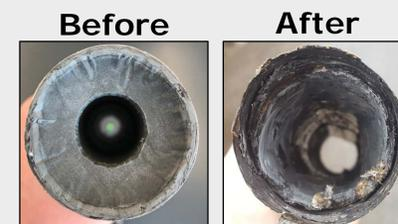
Figure 7: Finished fuel grain after spin casting and casting tube after a subscale test combustion.
