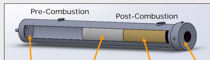
Figure 4: A rendition of the motor tube with important components labeled.
