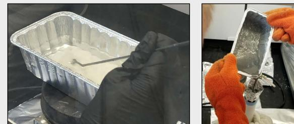
Figure 5: Melted wax with hexamine. Melting and mixing of components were done in a fume hood.
