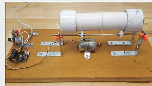
Figure 6: Spin casting system developed for fuel grain manufacturing.
