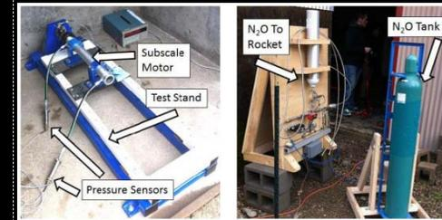
Figure 4. The fuel grains will be tested on a subscale motor at the OSU Propulsion Lab on the test stand above.
