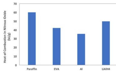
Figure 3. Paraffin wax shows the greatest energy of reaction with the oxidizer, followed by  $LiAlH_4$ . Both are key components of the fuel grain.
