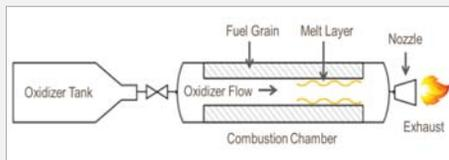
Figure 1. Basic components of a hybrid rocket. Oxidizer flows through the combustion chamber, reacts with the fuel grain, and exits through the nozzle.
