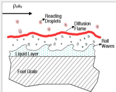
Figure 2. The melt layer, or liquid layer, produces droplets that increase the surface area of the fuel grain.
