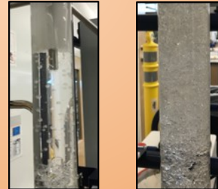
Figure 4. (Left) Snapshot at top of column, kerosene set at 80 mL/min. (Right) Snapshot at middle of column, kerosene set at 240 mL/min.
