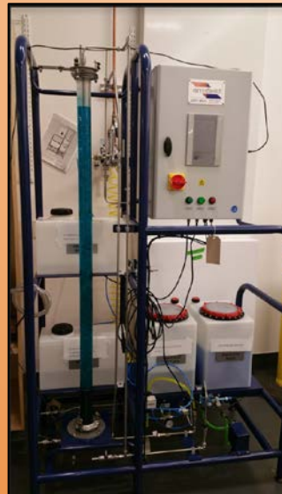
Figure 3. UOP5-MKII in Johnson Hall Laboratory. The unit included the extraction column, controller, and four reservoirs (feed, solvent, and two returns)
