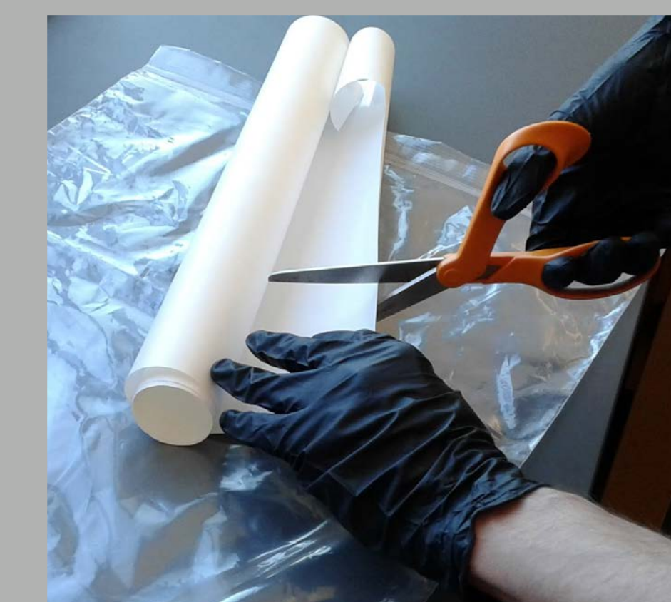
Figure 6 - Cutting from the roll of PDMS membrane provided to us by the kind folks at Membrane Technology and Research, Inc.
