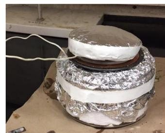
Figure 3: Experimental set-up for lithium nitrate salt testing. Lithium nitrate was placed in an insulated vessel, then water was placed on top to heat.
