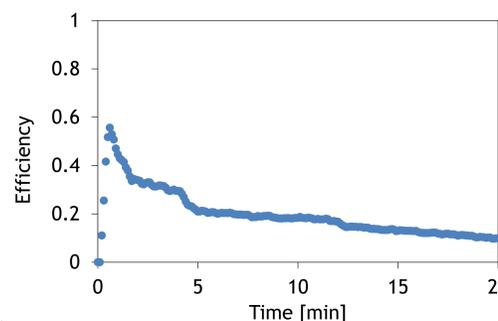
Figure 7: Efficiency of solar energy transferred to the aluminum block using the Fresnel lens. This was calculated using Equation 1. Based on the results of a single trial, the efficiency of the Fresnel lens is approximately 19% ± 9.4%.
