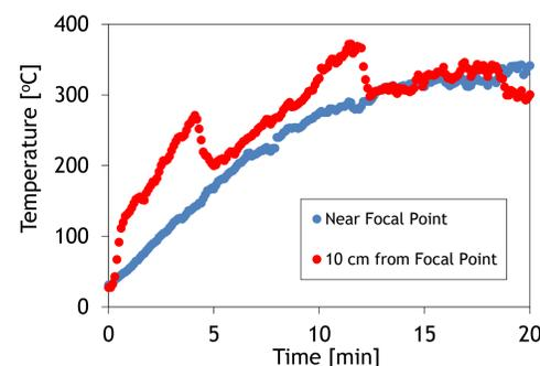
Figure 6: Temperature of a 437 g block of aluminum while being heated over 20 minutes using the Fresnel lens.
