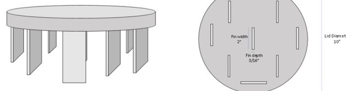
Figure 4: Lid design for the lithium nitrate container made from stainless steel due to its corrosion resistance. Fins extending into the salt increase heat transfer between the salt and the still.
