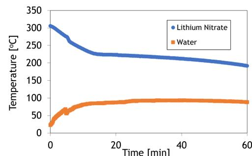
Figure 2: Heating of 25 mL of water over time using 280 g of lithium nitrate with a starting temperature of 310 °C. Experimental configuration below.
