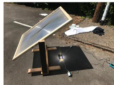
Figure 5: Experimental lens setup for heating aluminum block.
