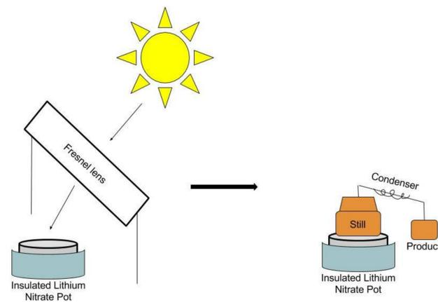
Figure 1: Process overview. A Fresnel lens melts lithium nitrate using solar energy, and that molten salt is used to power a batch distillation.
