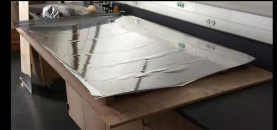
Figure 6. Current iteration of solar concentrator. Reflectivity will be improved through the application of an under layer of black paint to increase emissivity.
