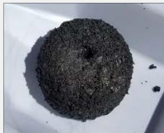
Figure 2. Salt vehicle made of activated carbon to house and preserve reaction surface area of the CaCl<sub>2</sub>.
