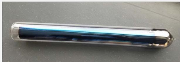
Figure 3. An evacuated tube dehydration chamber used to minimize heat loss to the surroundings.
