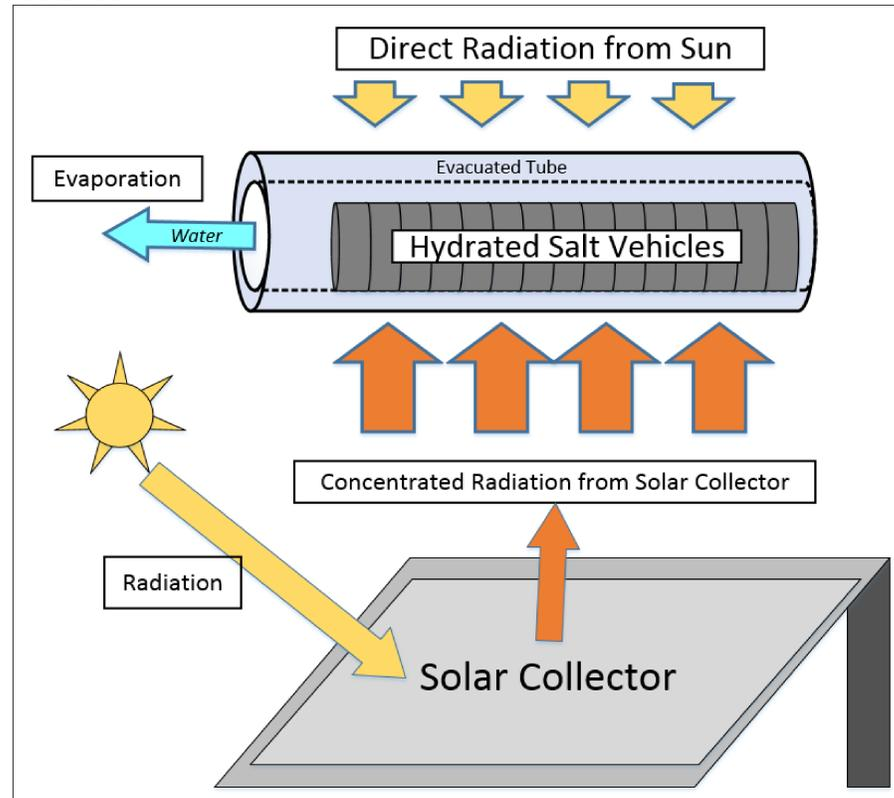
Figure 4. Evacuated tube schematic where incident solar rays are reflected from a solar collector to towards the tube, heating the salt vehicles within.
