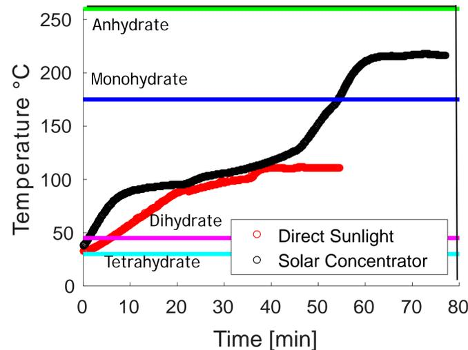
Figure 5. Temperatures achieved while testing a singular salt vehicle in the evacuated tube under direct sunlight compared to with the solar concentrator. The horizontal lines represent the hydration levels. Incident radiation during testing averaged approximately 850 W/m<sup>2</sup>.
