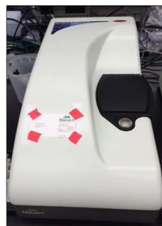
The Zetasizer measures the hydrodynamic diameter of the emulsion droplets by dynamic light scattering. The frequency of size measurements is displayed as a function of intensity. To reduce the polydispersity index (PDI), larger emulsion droplets are removed by a 0.2 μm syringe filter and measured again.
