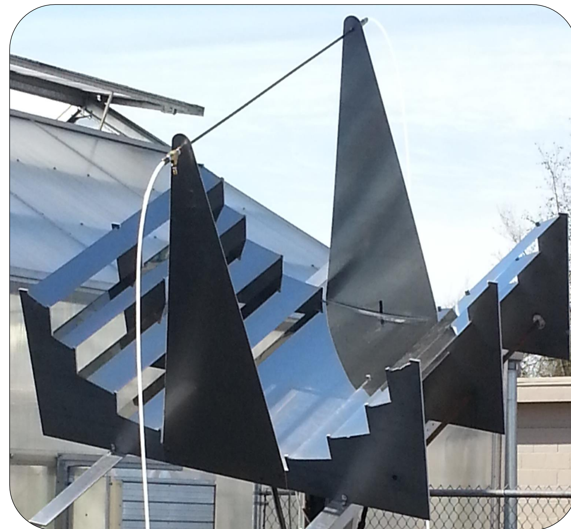
Figure 1: The SRSC reflects light with a series of curved panels onto a collector rod that has water flowing through at a known flow rate, with monitored input and output temperatures.
