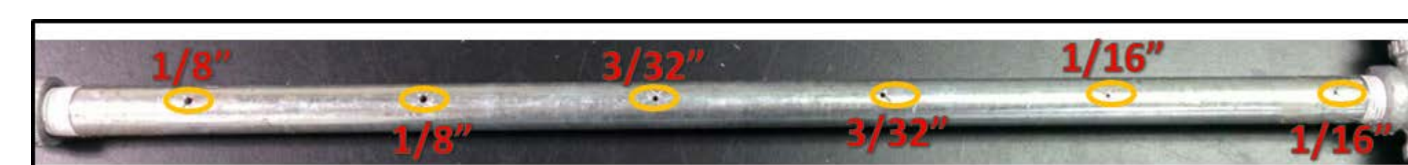
Fig. 4: Hole diameters along each pipe.
