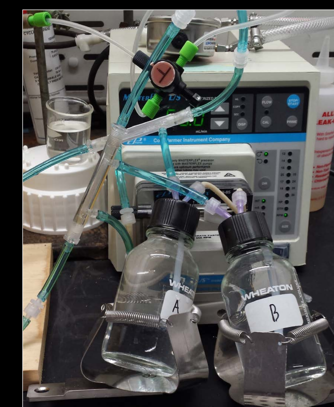
Figure 7. Separate cell culture solutions were pumped through two membrane units. The solutions are contracted with 29% methane and 71% air via silicone membrane module to stimulate cell growth. Liquid flowrate was kept low to prevent shearing of the biofilm.
