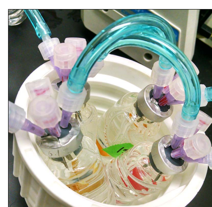
Figure 3. Semi-batch reactors growing MOT OB3b in stagnant media. Reactors were inoculated with 0.1, 1, and 10 mg/L cell concentration, and were ran for ~4 days.
