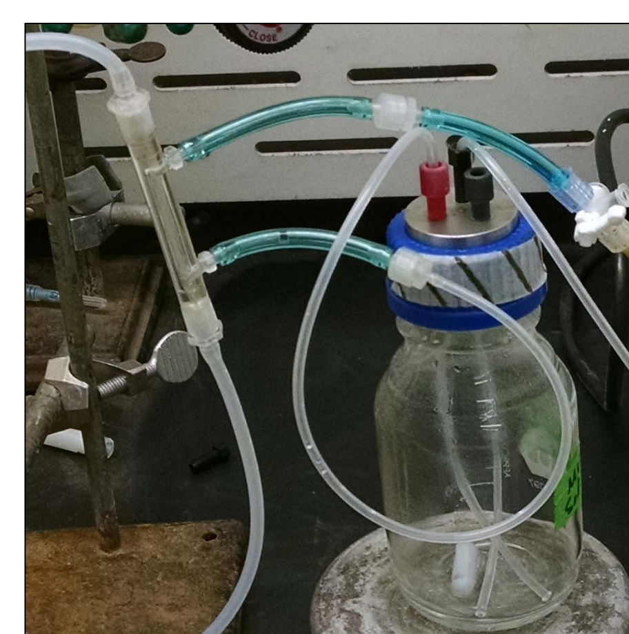
Figure 2. Membrane module with 10 cm 2 of interfacial surface area 2 was ran for 40 min, with pure oxygen at ~2 psig flowing at 10 mL/min on tube side of the unit, saturating ~200 mL of water recirculating through shell side.
