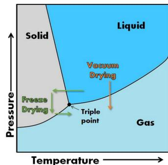
Freeze drying, or lyophilization, takes advantage of the process of sublimation. First samples are frozen to -80 °C, and then they are placed in a 50 mTorr vacuum chamber in which ice crystals change directly into water vapor, bypassing the liquid phase. Vacuum drying evaporates water by reducing pressure, leaving dried reagents in samples. These methods generally increase shelf life of perishable materials, and makes transport easier.
