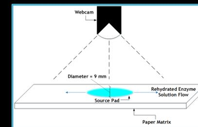
Webcam method for observing enzyme release from source pad. MATLAB analysis can model enzyme quantity exiting pad over time.
