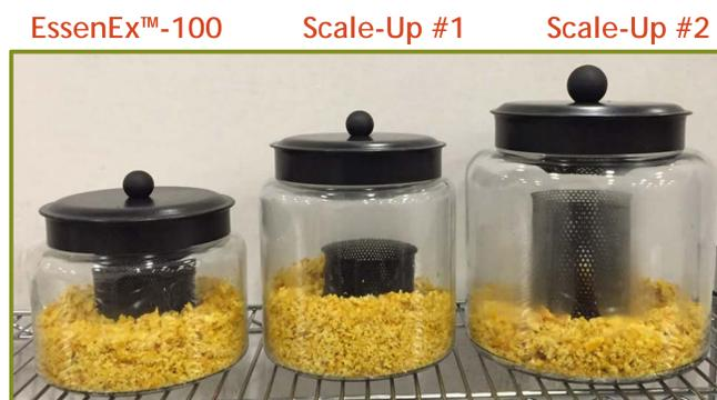
Fig.1: Size comparison of the EssenEx™-100, Scale-Up #1, and Scale-Up #2. All units contain 400 g of chopped orange peel.
