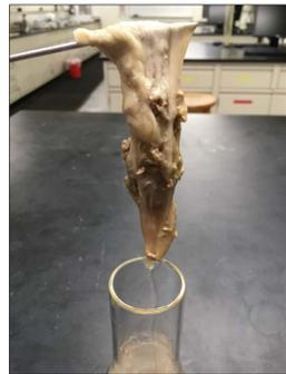
Cells form large aggregates which can clog drainage pipes and accumulate on sensors. A settling tank should be used to decrease filtration time and energy requirements.
