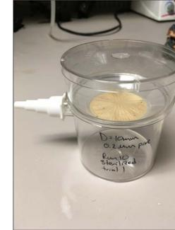
A 50 mL sample of broth from Run 10 was filtered to estimate filtration time in the full scale process. A Nalgene filter unit with 50 mm diameter and 0.2 μm pore size was used. The filtration time was 1 hour.
