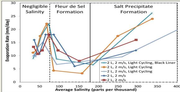
Graph 2: Evaporation rate with respect to salinity for several trials. Fleur de Sel was observed forming from 75 to 175 parts per thousand (ppt), while solid salt precipitated at above 175 ppt. Both regimes are characterized by a change in evaporation rate.
