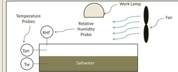
Figure 3: Schematic of the bench scale apparatus used for initial determination of evaporation rate and dependencies on the parameters shown.
