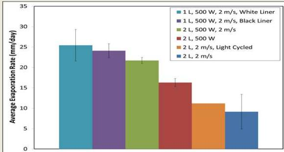
Graph 1: Average evaporation rate six configurations where volume, light, wind speed, and liner were varied as indicated in the legend. Error bars for one standard deviation with further analysis to come.
