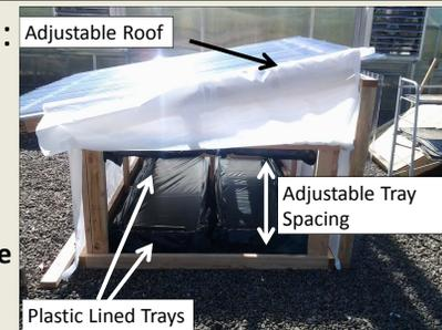
Figure 4: Adjustable scale model currently being used for testing. Structure build by the team.
