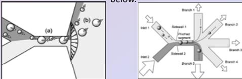
**Figure 1:** Pinch point (a) particles enter separate flow regimes leading to fractionation of particles (b). **Figure 2:** Particles separated into different channels.
