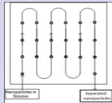
1 m channel length designed to allow sufficient flow disruption pockets and desired separation.
