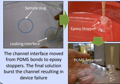
The channel interface moved from PDMS bonds to epoxy stoppers. The final solution burst the channel resulting in device failure
