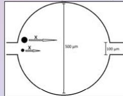
Channel feature dimensions demonstrates larger particles traveling further during deceleration than smaller particles
