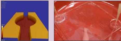
Microchannel pocket feature designed to cause acceleration and deceleration unique to particle size. Pocket features increase separation of nanoparticles per Stokes' drag force
