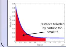
The model showed that little to no separation occurs using the chromatography microchannel design.
