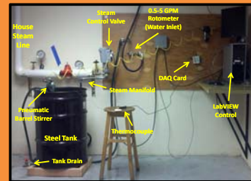
Figures: (on the left) A P&ID (piping and instrumentation diagram) with dimensions. (above) The actual lab equipment constructed in Gleeson's basement.
