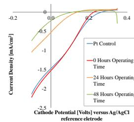
Figure 4. Degradation of Fe/EDTA over a period of time. The first test was comparable to platinum.
