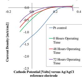
Figure 3. Degradation of nitrogen doped graphene over 3 days. The catalyst degrades quickly in a short time.
