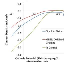
Figure 6. Graphite oxide performed better when used in catalysts than the mildly oxidized graphite.
