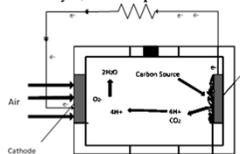
Figure 1. The chemical process of a MFC. The entire reaction occurs spontaneously.
