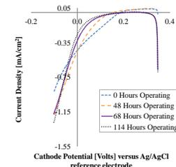
Figure 5. The nitrogen doped graphene with cobalt oxide nanocrystals catalyst did not degrade as quickly as other catalysts
