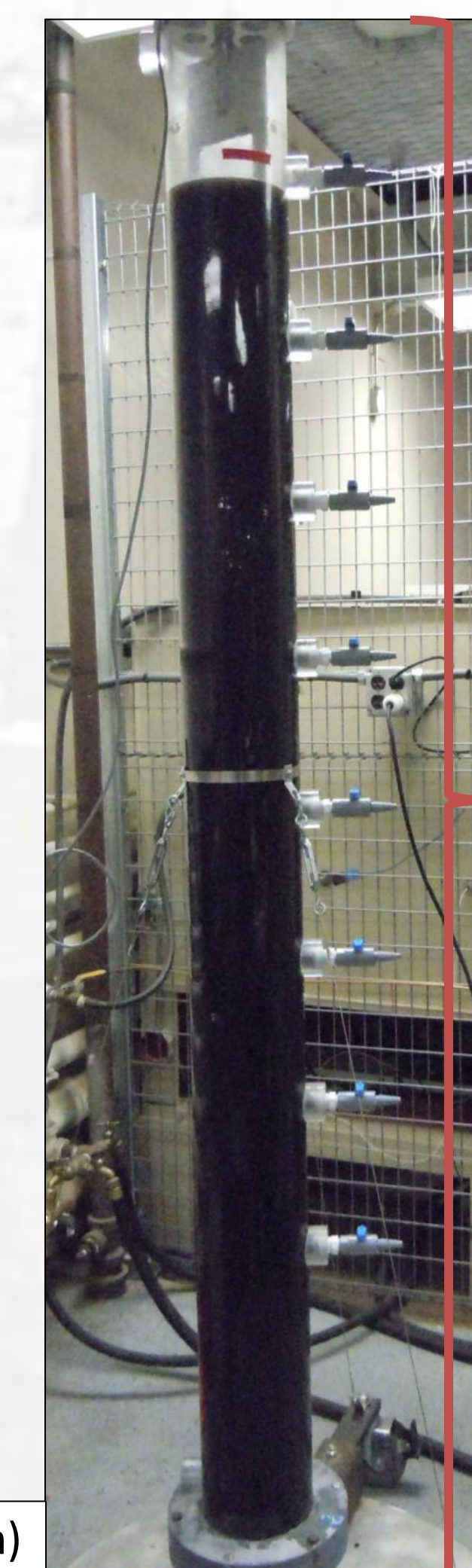
Scaled up settling column (2 m)
