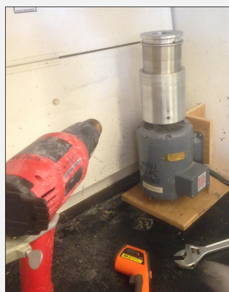
Figure 3: Solution of CNC and DMAC is left in rotary caster with a heat gun applied to maintain 60 °C for four hours
